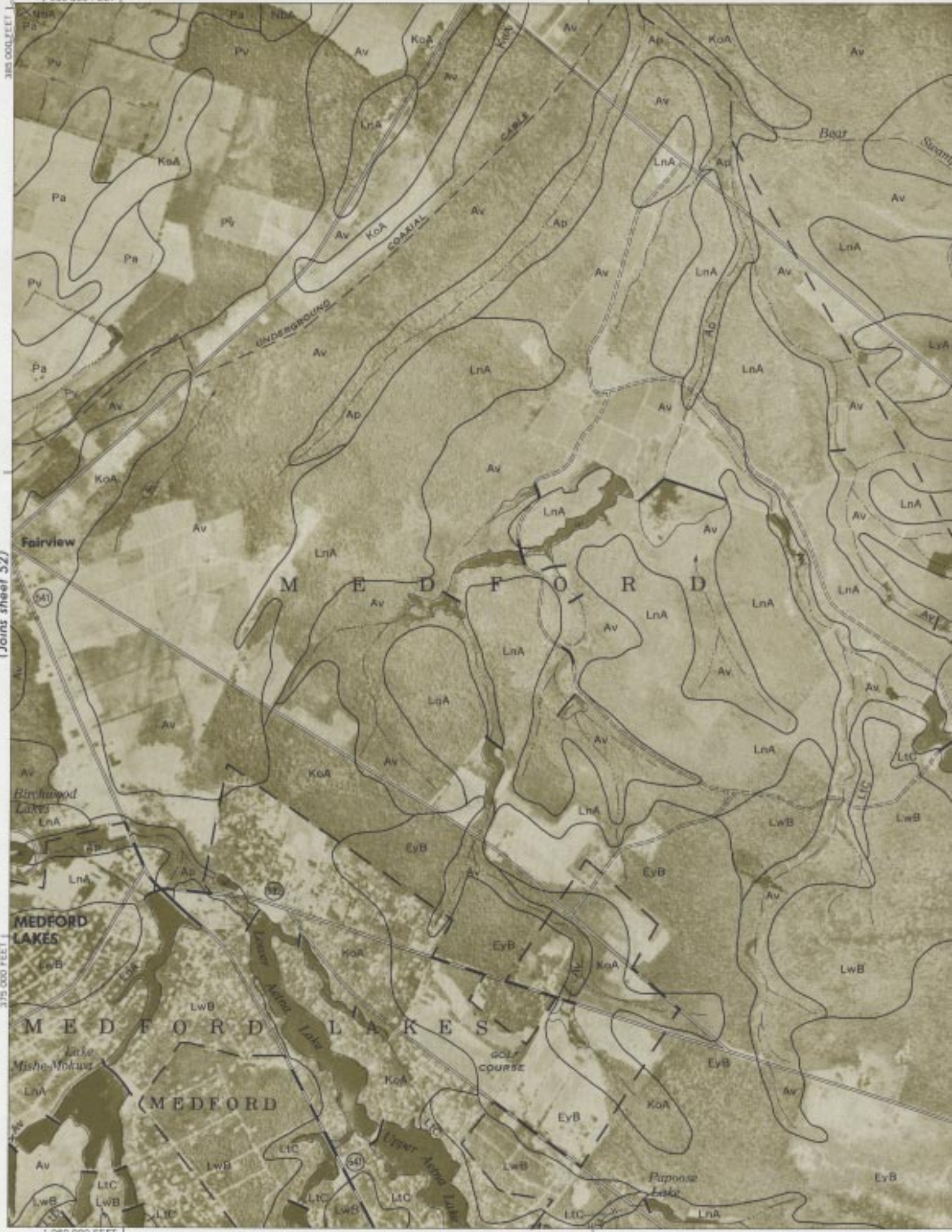
This map is one of a set compiled in 1970 as part of a soil survey by the United States Department of Agriculture, Soil Conservation Service, and the New Jersey Agricultural Experiment Station. Photo base from 1963 aerial photographs. 5,000-foot grid ticks based on New Jersey plane coordinate system. 1927 North American datum.
